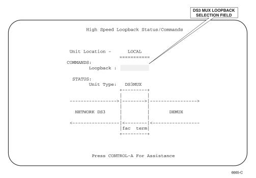
Note: Do not perform a DS3 loopback when the Soneplex Broadband chassis is connected to a DS3 CAM unit in the Soneplex CCAS system.
